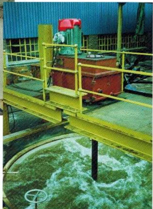
Final test on Series 4000 in 5m Dia test tank
