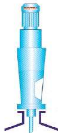
Flange Mount with Bearing Cartridge for High Tank Pressure Application
