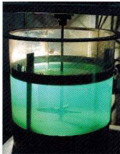
Solid suspension test work on Copper leaching application.
