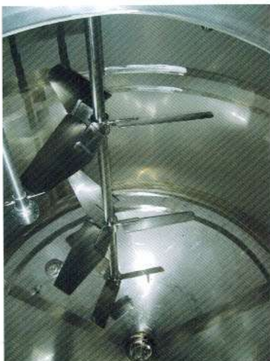
Multi stage fermenter hygienic designed surfaces for CIP processes
