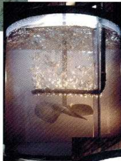
New gas dispersion impellers and sparge rings under test
