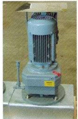
Series 1000 with weather protection and VVVF control
